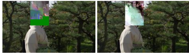
(a) TNE-HEVC PSNR1=10.95, (b) TSE-HEVC PSNR1=7.78, PSNR2=42.07, PSNR3= 21.15(dB) PSNR2=42.07, PSNR3=18.01 (dB)
